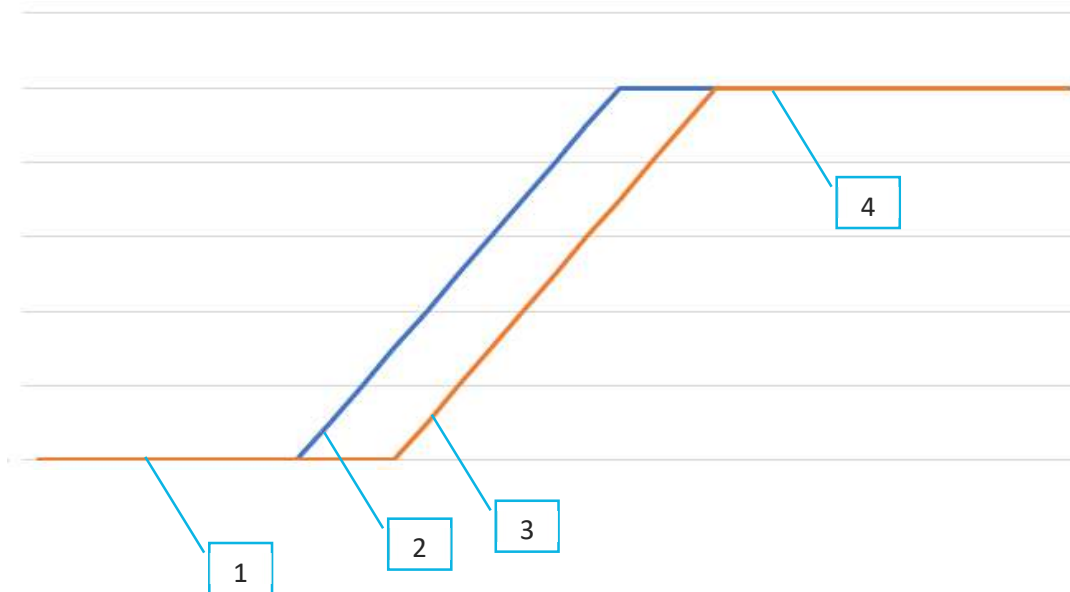
Figure 18.- Commissioning diagram (Temperature variation of the hot Surface in contact with the Thermoelectric generator module- blue line; InduEye® LeakSense/TempSense module charging process-orange line).
